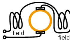
Uncompensated series AC motor.
