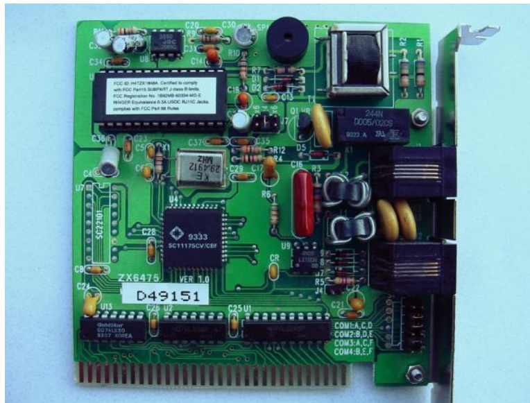
Printed circuit board mounted audio impedance matching transformer, top right.
