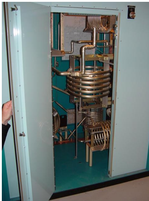
High power inductors formed from hollow tubes.
