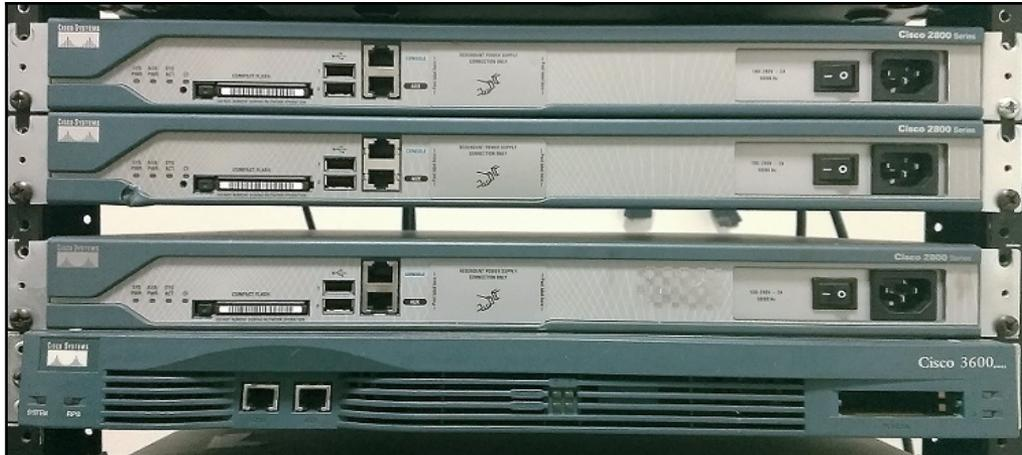
Figure 1.15. Stack of Cisco routers
