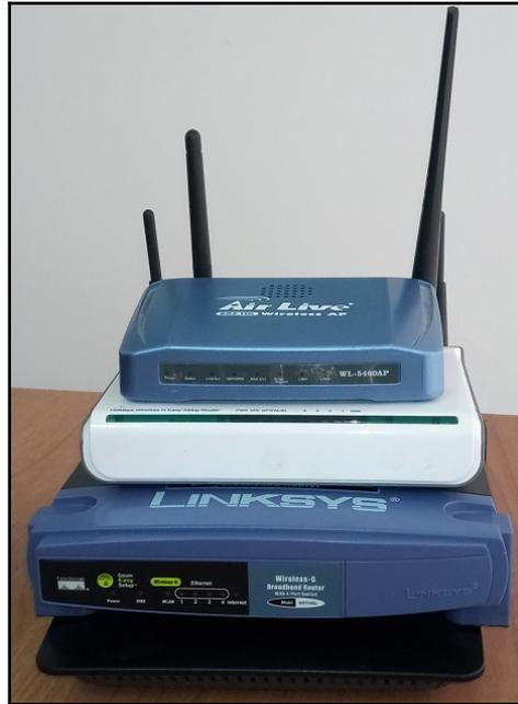
Figure 1.17. Stack of access points (APs)
