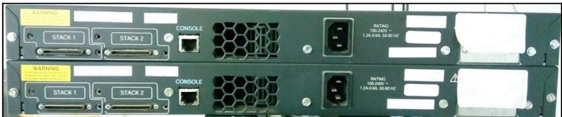
Figure 3.13. The rear of stackable configuration switches with stack ports
