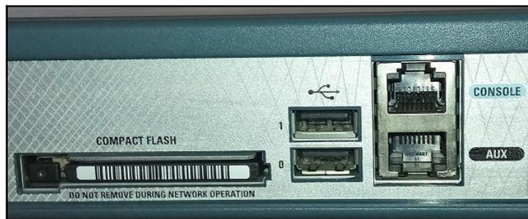
Figure 7.19. USB ports on a front panel of a router
