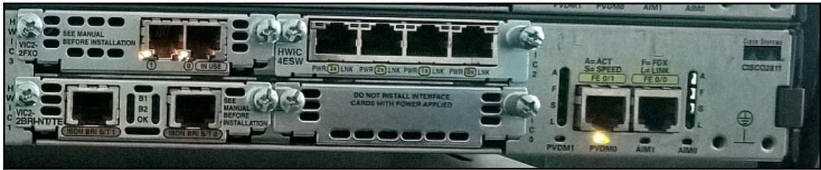
Figure 5.16. Router's interfaces and ports
