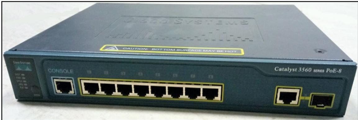
Figure 3.10. Power over Ethernet (PoE) multi-layer switch
