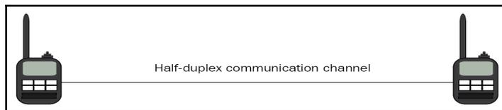
Figure 2.8. Radio communication, which represents a half-duplex communication channel
