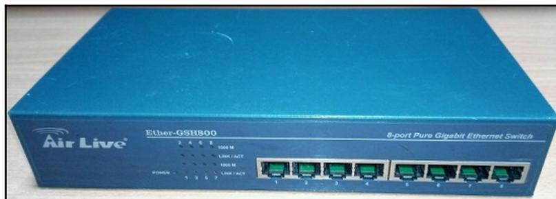
Figure 3.1. Unmanaged switch
