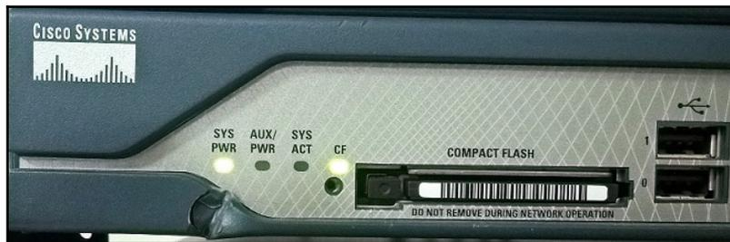
Figure 6.1. LED indicators on router's front panel
