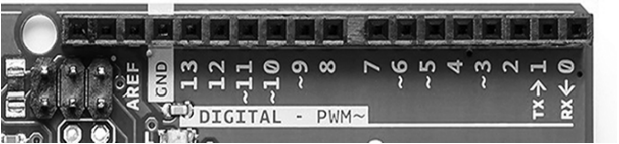
Figure 2-5: The digital input/output pins
