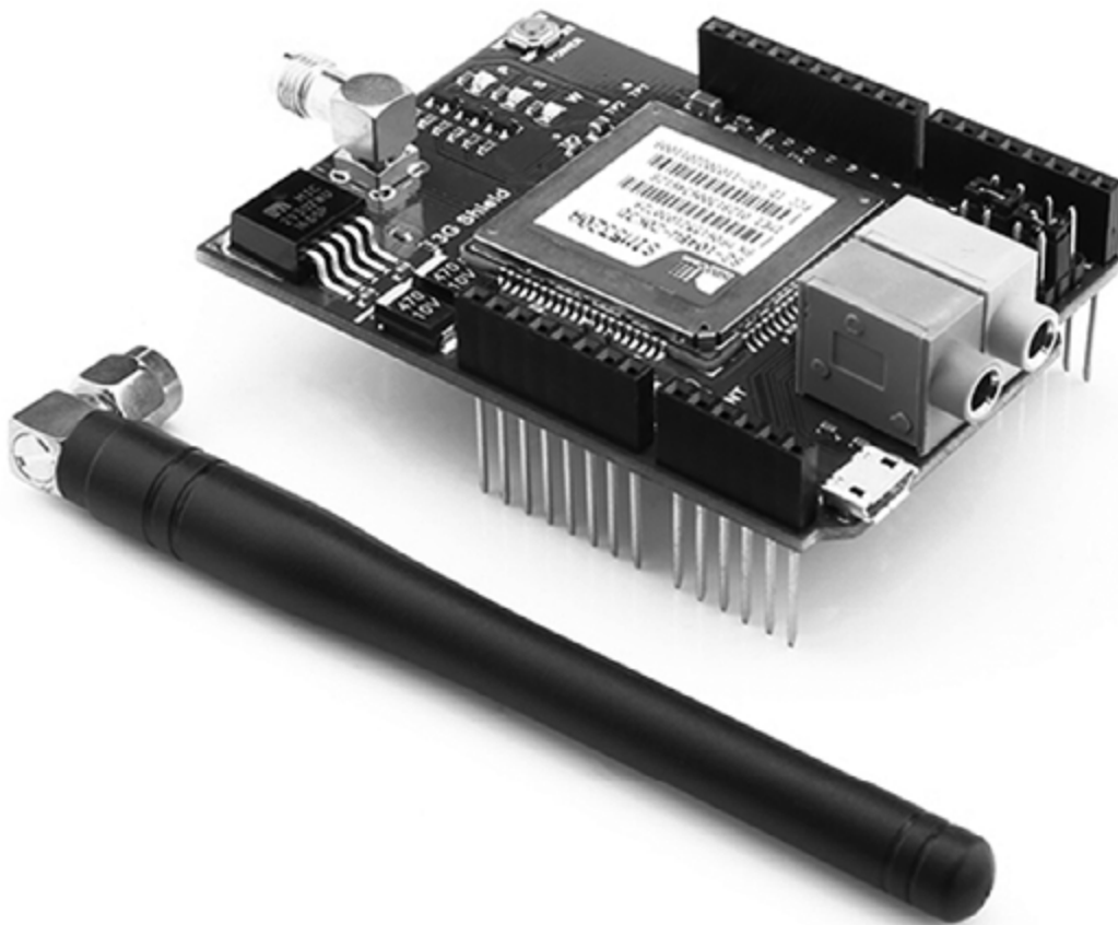
Figure 22-1: 3G shield with antenna attached
