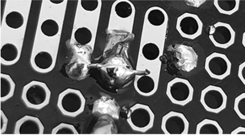
Figure 7-11: A solder bridge
