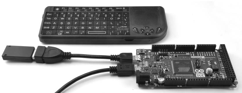
Figure 13-3 Arduino Due with a Micro USB OTG Host Cable and keyboard.
