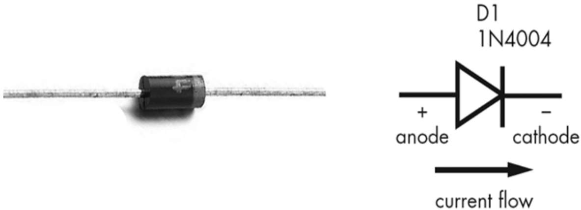
Figure 3-17 : A 1N4004-type rectifier diode
