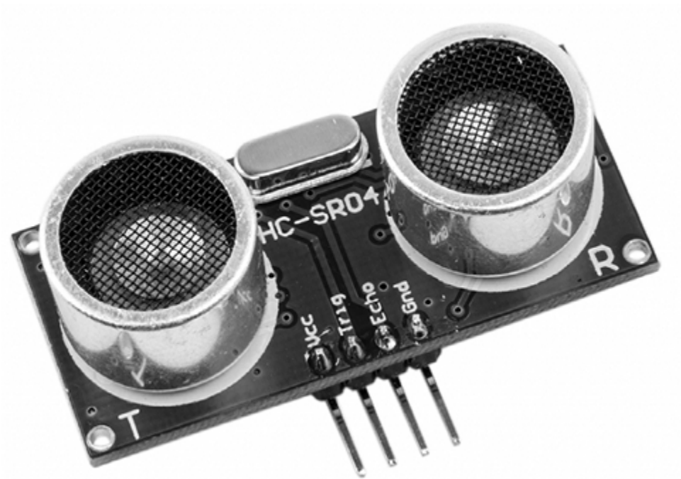
Figure 14-27: The HC-SR04 ultrasonic distance sensor
