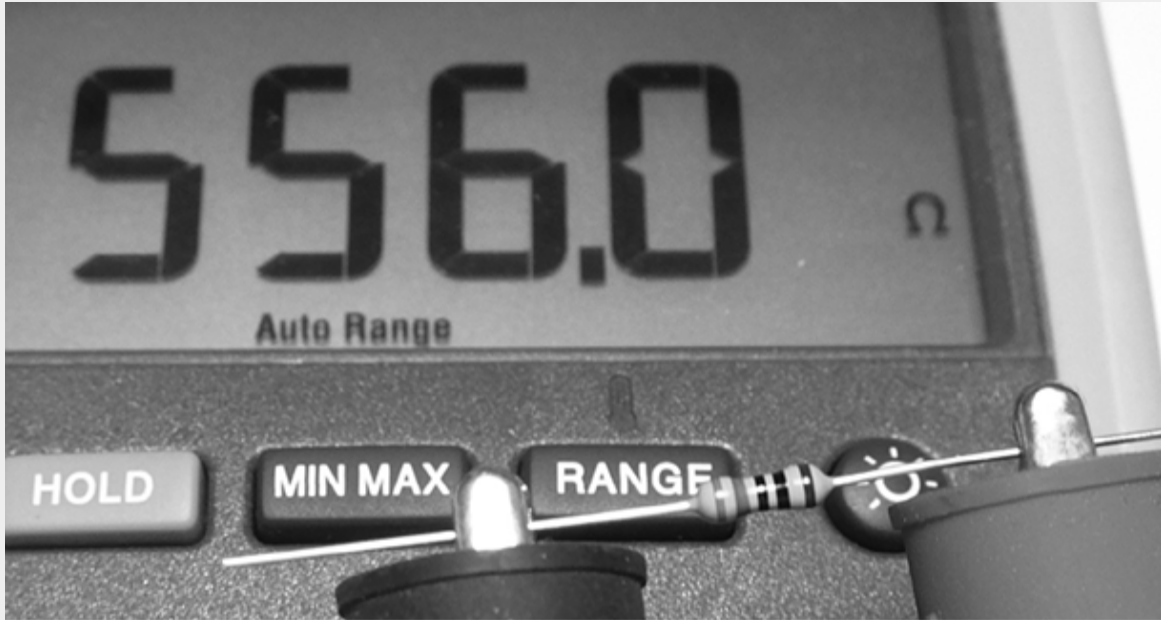
Figure 3-4 : A multimeter measuring a 560 \Omega , 1 percent tolerance resistor
