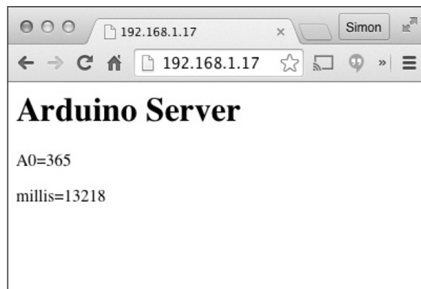
Figure 10.4 A simple Arduino server example .
