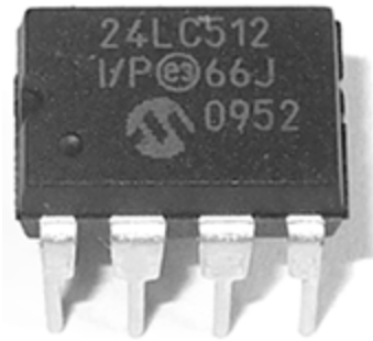
Figure 19-4: Microchip Technology's 24LC512 EEPROM
