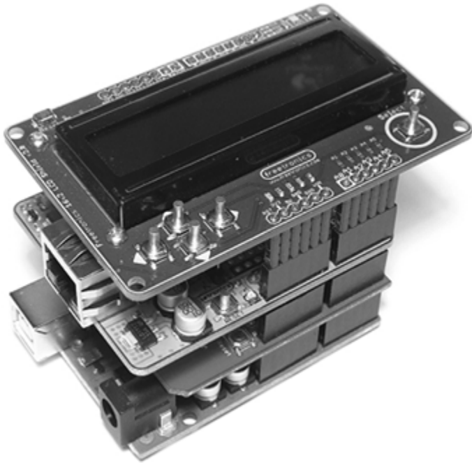
Figure 7-4: Three stacked shields with an Arduino Uno
