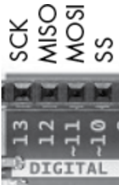
Figure 19-10 : SPI pins on an Arduino Uno
