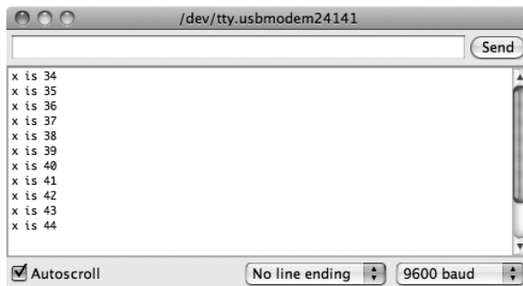
Figure 9-7 Serial Monitor output for Arduino to Arduino over I2C.
