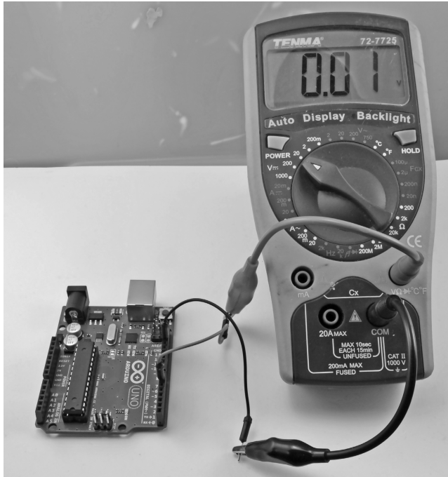
Figure 1-18 Measuring the output voltage.
