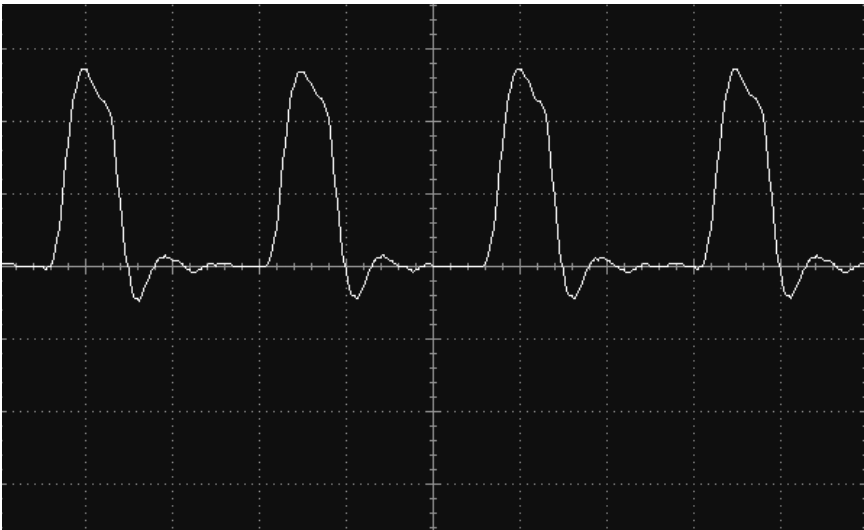
Figure 5-5 Generating a 4-MHz signal with an Arduino.
