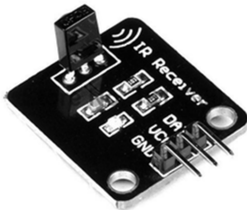
Figure 17-2: A prewired IR receiver module
