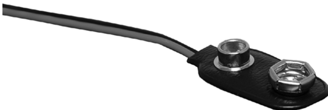
Figure 14-16: A battery cable used to connect the battery holder to the Arduino
