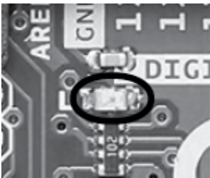
Figure 2-11: The LED on the Arduino board, next to the capital L
