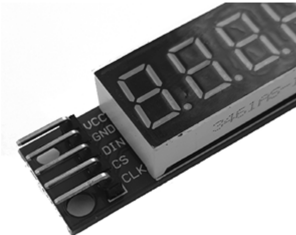
Figure 8-4: Inline header pins connected to an eight-digit LED module
