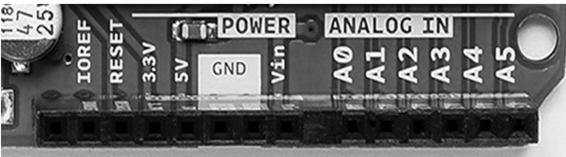
Figure 2-4: The power and analog sockets
