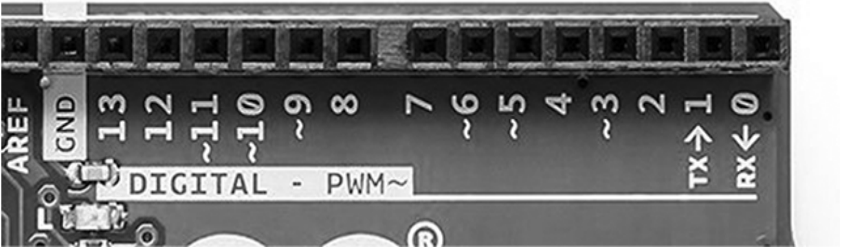
Figure 3-15: The PWM pins are marked with a tilde (~).
