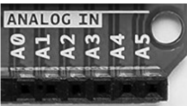
Figure 4-30: Analog inputs on the Arduino Uno
