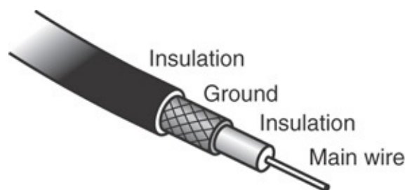
FIGURE 5.2 Coaxial cabling
