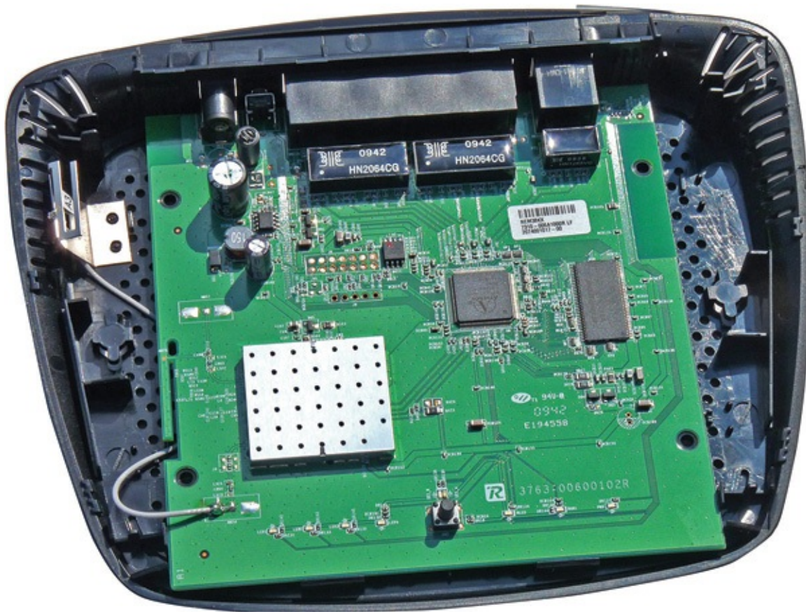
FIGURE 6.3 The antenna is the wire and metal component on the left
