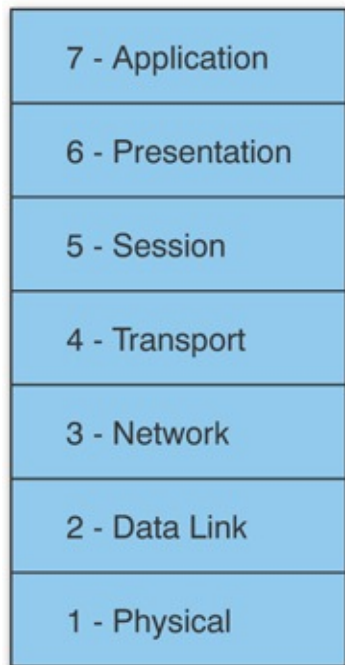
FIGURE 2.1 The OSI seven-layer model
