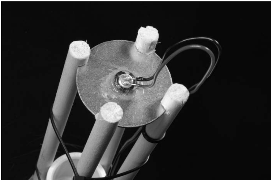
Figure 4-19: With the microphone cartridge in place.
