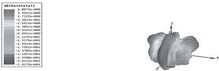
FIGURE 1.12 (See color insert.) Gain plot of the two-element antenna array of mitered bend feed network.
