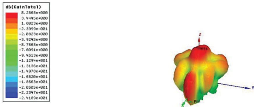
FIGURE 2.11 Gain plot of the two-element antenna array of quarter-wave feed network.
