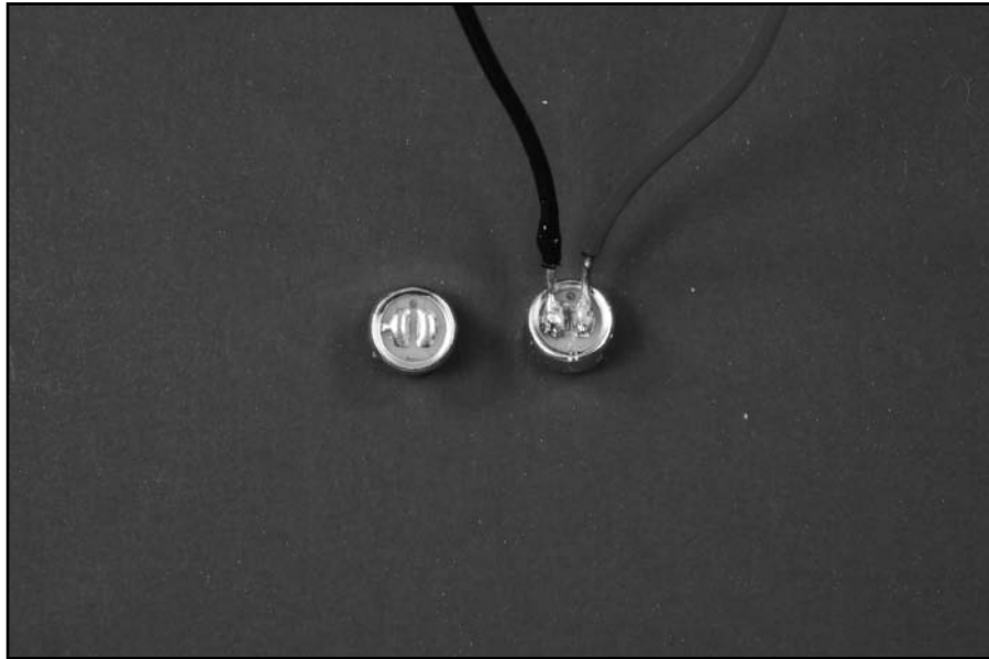
Figure 4-14: Soldering to flat contact pads.
