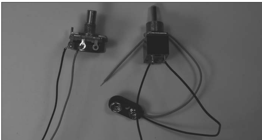
Figure 9-12: Solder wires to the on/off switch and the potenti- ometer.
