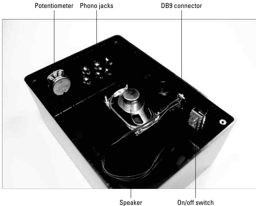
Figure 7-11: Mount components on the box.
