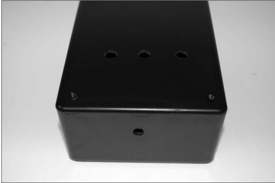
Figure 11-14: Drill holes for the LED and switches.
