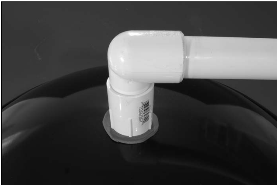
Figure 6-11: Fittings assembled on the parabolic dish.
