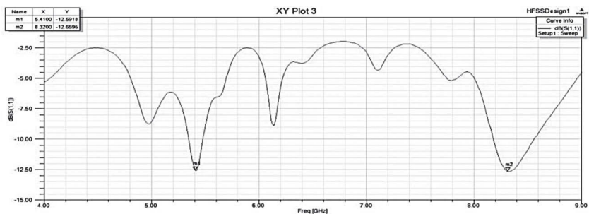
FIGURE 2.7 Reflection coefficient curve of the two-element antenna array of quarter-wave feed network.
