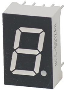
Figure 5.10.2: Seven-segment display (CC BY-NC-SA; BC Industry Training Authority)
