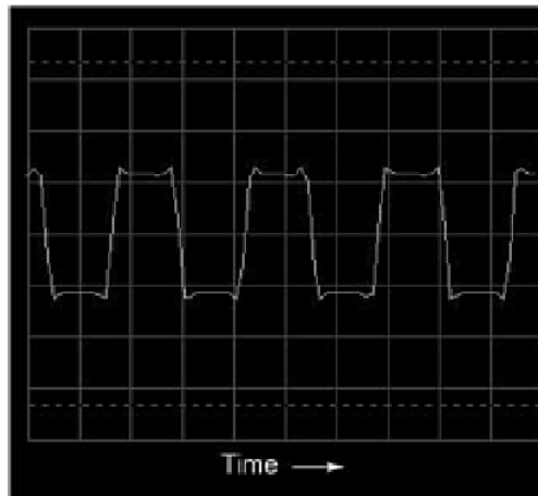
Oscilloscope time-domain display of a square wave
