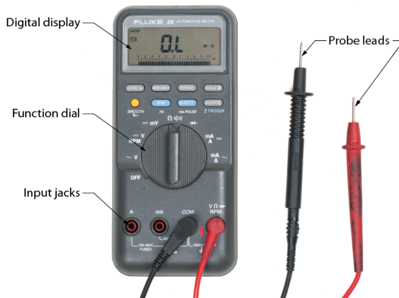
Figure 12.3.1: Typical DMM (CC BY-NC-SA; BC Industry Training Authority)
