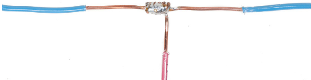
Figure 9.2.2: Tap joint (CC BY-NC-SA; BC Industry Training Authority)
