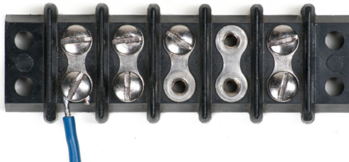
Figure 9.3.2: Proper installation under terminal screw (CC BY-NC-SA; BC Industry Training Authority)
