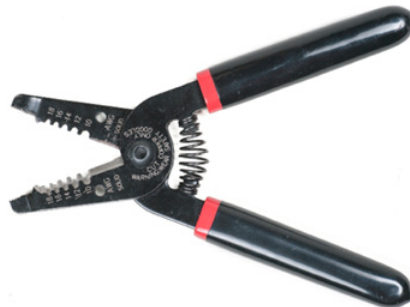
Figure 9.1.3: Wire strippers (CC BY-NC-SA; BC Industry Training Authority)
