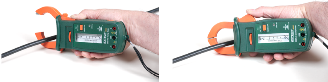
Figure 12.5.3: Using clamp-on ammeter (CC BY-NC-SA; BC Industry Training Authority).
